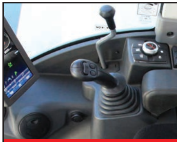
Hydraulic Pilot Controls
