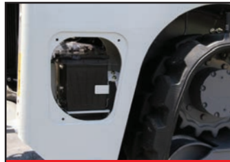
Battery Access Panel
