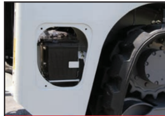
Battery Access Panel
