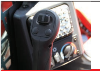
Pilot Operated Controls
