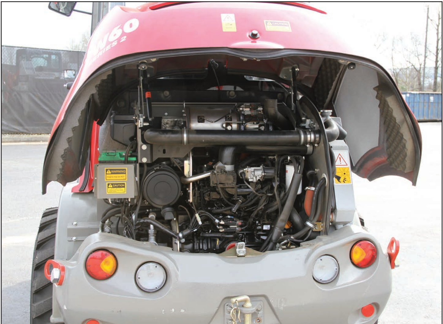
Large Lockable Rear Service Hood Provides Outstanding Service and Maintenance Access
