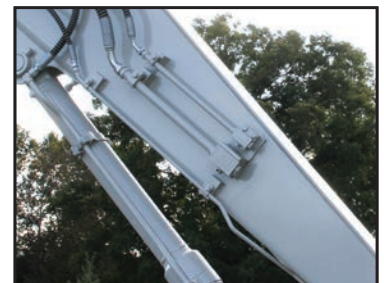
Auxiliary Hydraulic Lines
