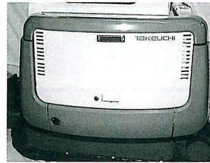
Wrap-around counterweight protects engine compartment.
