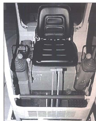
Deluxe operator's compartment with joystick servo controls for precise and comfortable machine operation.
