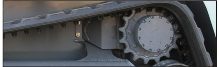
All Takeuchi track loaders feature double reduction planetary drives that generate exceptional traction force allowing the machine to power through the most demanding applications. Drive lines are protected by a heavy gauge steel guard that keeps them from being damaged when working or cleaning the machine.
