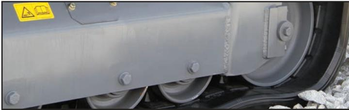
Several different track systems can be found on Takeuchi track loaders. The TL8 features steel on steel contact between the rollers and mandrels allowing abrasive material to be crushed or expelled from the track system. The TL10V2, TL12R2 and TL12V2 have a quiet ride track system that allows the rollers to ride along a rubber contact pad reducing noise and vibration levels.
