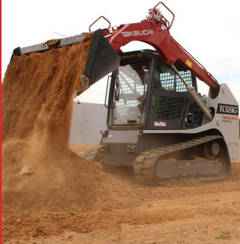
Radial lift machines feature a single arm pivot point and have higher breakout forces making them ideal for tough excavating and grading applications. They also have excellent mid-height reach which is well suited to loading and unloading flatbed trucks.
